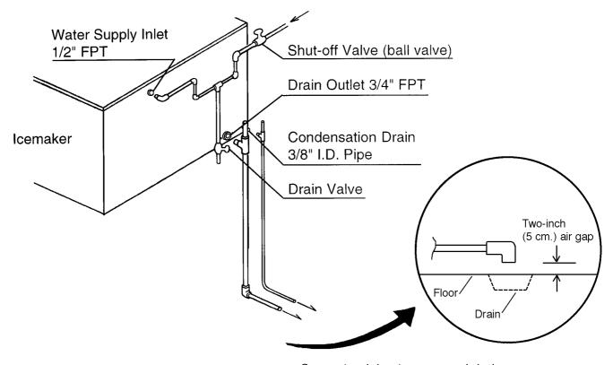
Separate piping to approved drain. Leave a two-inch (5 cm.) vertical air gap between the end of each pipe and the drain.
